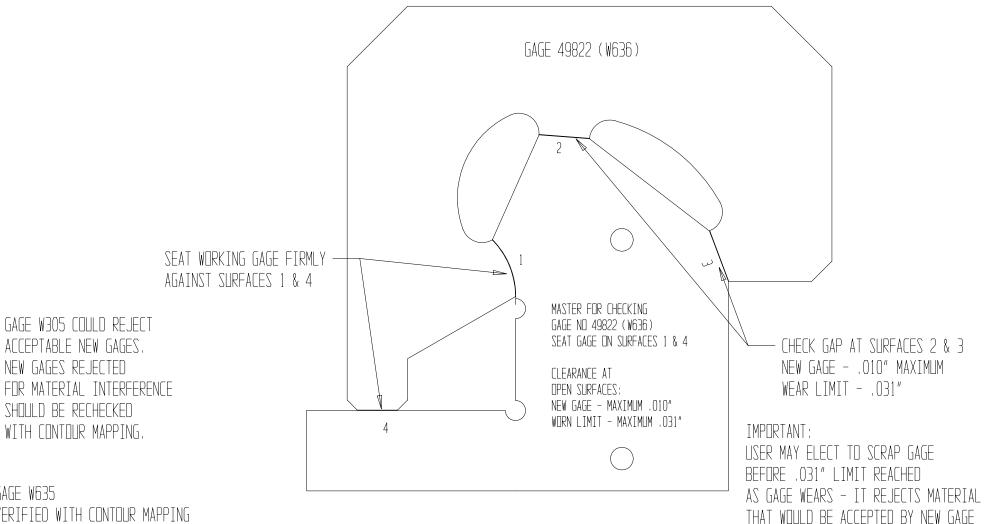
GAGE W635 VERIFIED WITH CONTOUR MAPPING MAX MANUFACTURE DEVIATION: .005" MAX RECERTIFICATION DEVIATION: .015"
