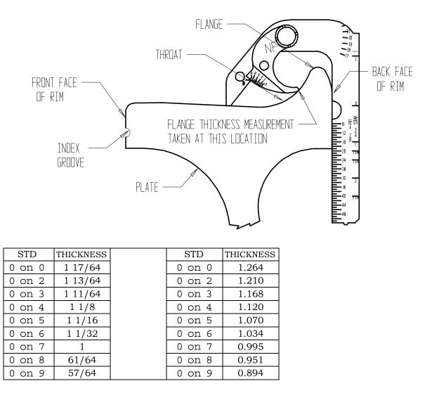
PLACE WHEEL GAGE ON BACK FACE OF RIM WITH HOOK ON THE TREAD OF THE WHEEL. ENSURE THAT GAGE IS FLUSH WITH THE BACK FACE OF THE RIM AND THE HOOK IS IN CONTACT WITH THE TREAD ON THE WHEE. MOVE GAGE FINGER TO THE FLANGE SO IT IS TOUCHING AND THEN READ MEASUREMENTS ON THE FINGER SCALE TO THE "0" READING ON THE HOOK PORTION OF THE WHEEL GAGE.
